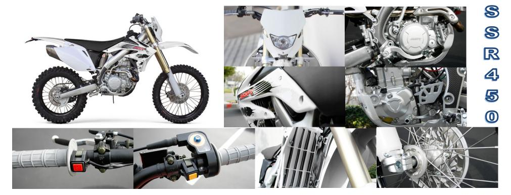
Engine Type 449CC, 4 Stroke Single Cylinder
